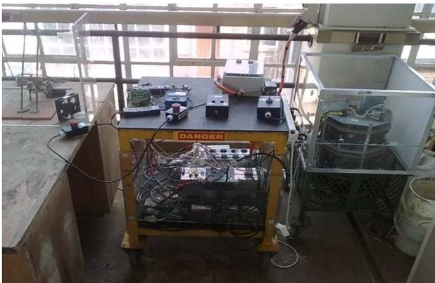
Figure 1. CSIR in-house, high-voltage, AC-based test rig (60 kHz).
